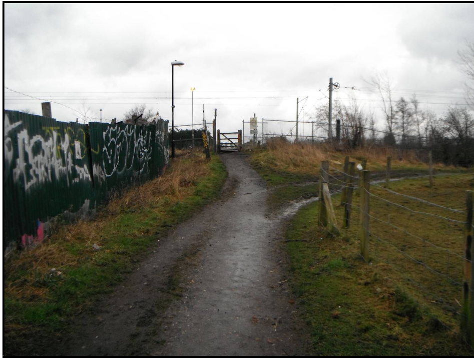
Figure 28: The un-metalled access track that runs in parallel with the railway shows signs of vehicular use. This is most likely to gain access to the adjacent fields. Horses were in the fields at the time of the site visit. Vehicular use of the access track is an additional risk for users of the crossing. The Census of Rail and Pedestrian Users records daily use of the crossing by someone with a wheelbarrow moving horse feed to this side of the railway.
